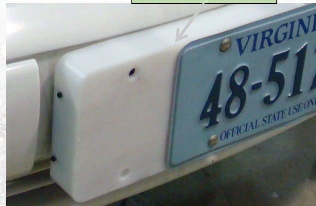
Front Radar Assembly
