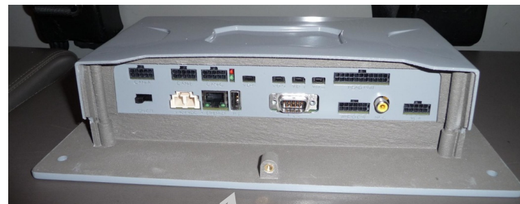
Front Radar Assembly
