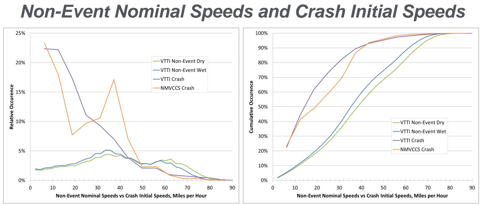
Velocity distributions are compared between wet and dry conditions and between normal "non-event" driving and crash events. This data is then compared to the crash data from NHTSA's NMVCCS database. The model is simulating a wet braking scenario, so the wet non-event speed distribution was used.
