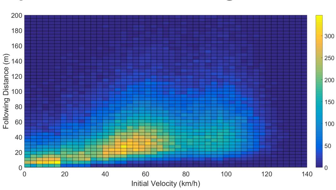
Based on a bivariate distribution for following distance and velocity, a representative distribution of following distances can be found for a selected velocity.
