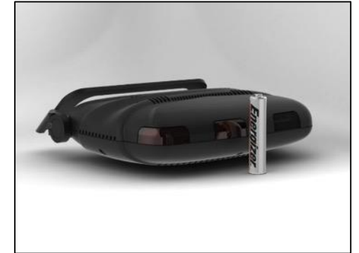
MiniDAS as compared to a standard AA battery.
