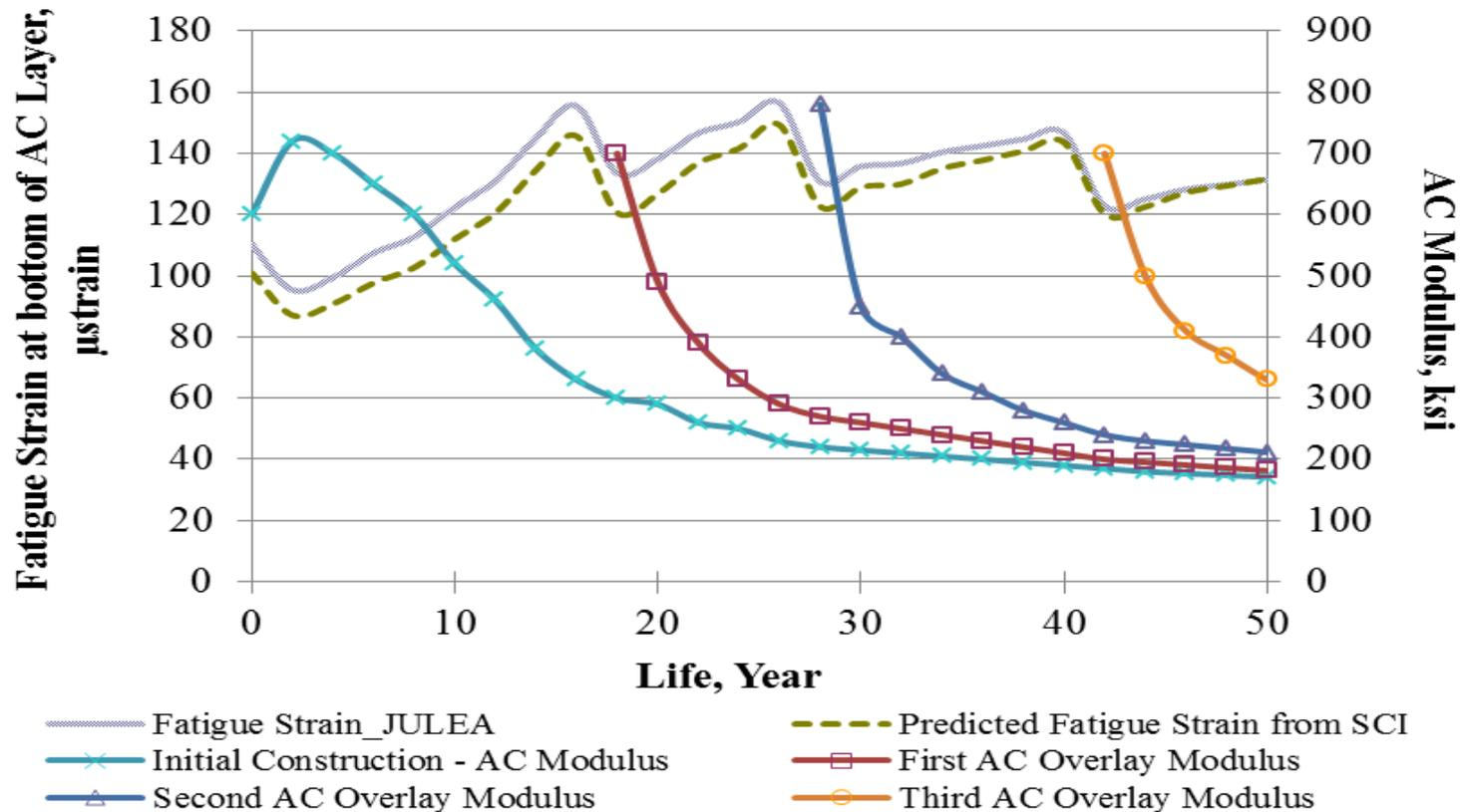
Fatigue strain can be a continuous structural indicator even after successive treatments.
