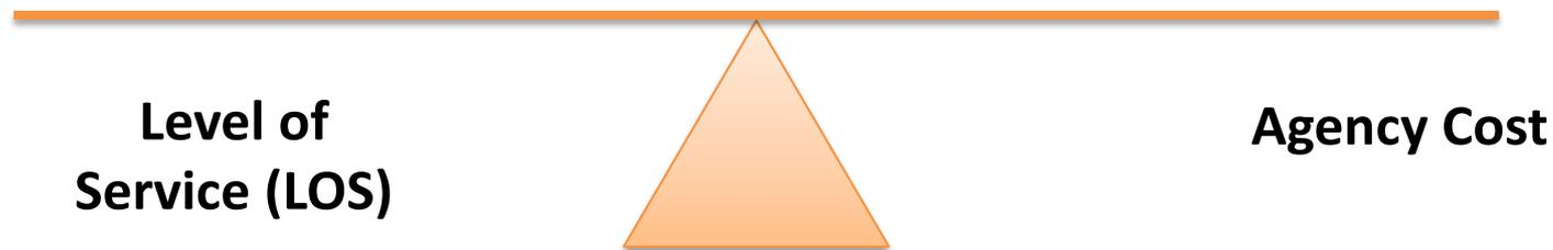
Objective is to maintain pavement at or above acceptable LOS to user at minimum practical cost over the lifecycle of asset
