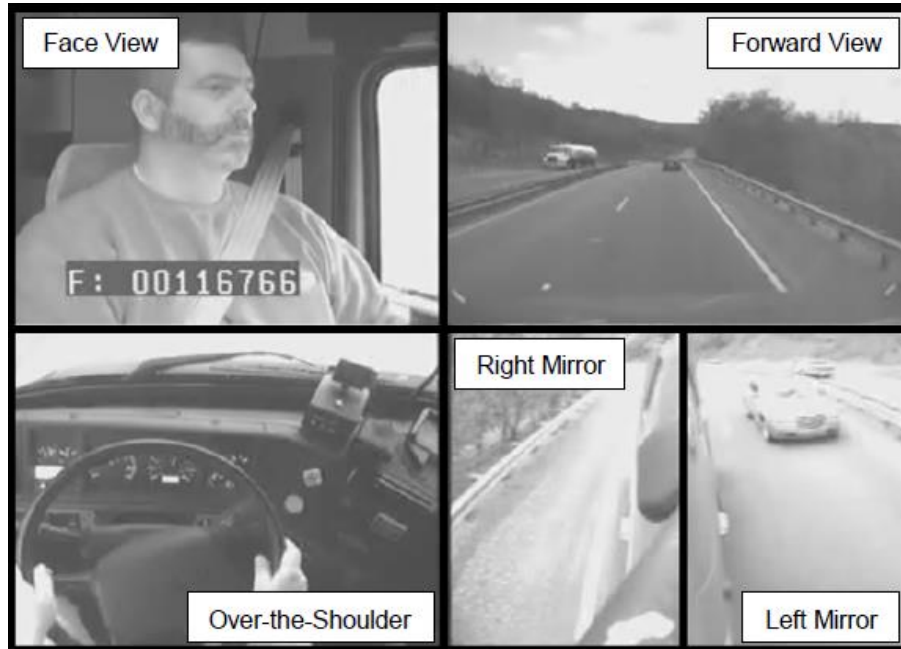
Figure 1. Photo. Five Camera Images Multiplexed Into a Single Image. The driver depicted is a VTTI employee.
