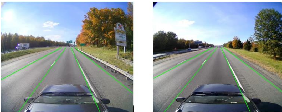
Figure 77. Image overlay. The images show the application of the CLRRerNET algorithm to ADS CONOPS Cross-Country data to measure shoulder width.
