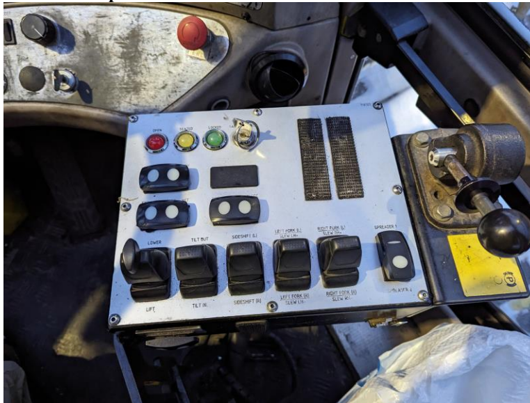
Figure 27. Photo. Mast and pick control panel.
