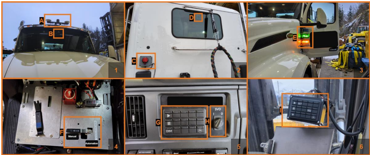
Figure 22. Photo. The primary ADS equipment. See Table 8 for equipment descriptions.
