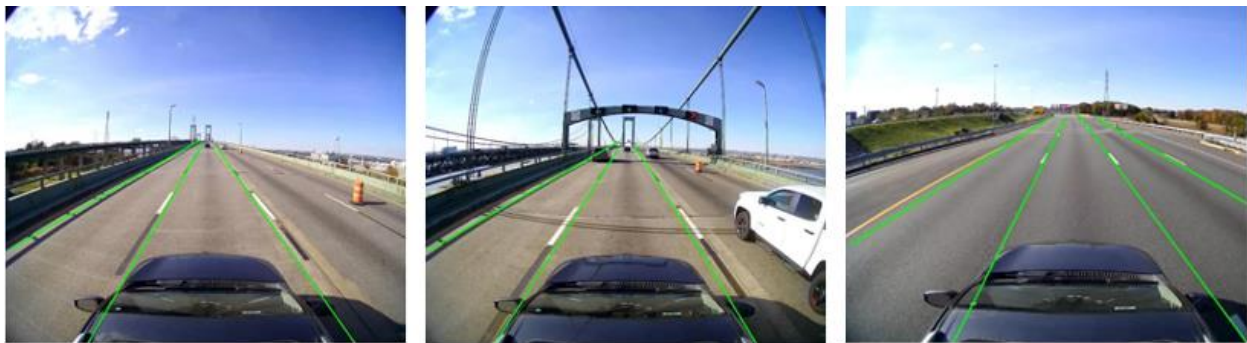
Figure 78. Image overlay. The images show the application of the CLRerNET algorithm to ADS CONOPS Cross-Country data to measure lane lines.
