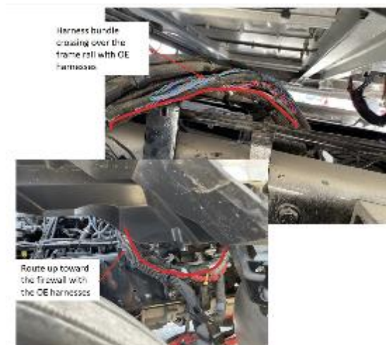
21. Route and on right and XXX up to the treadle valve
