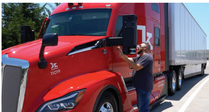
Figure 3. CVSA certified ADS inspector checking sensors on a Kodiak ADS-equipped CMV
