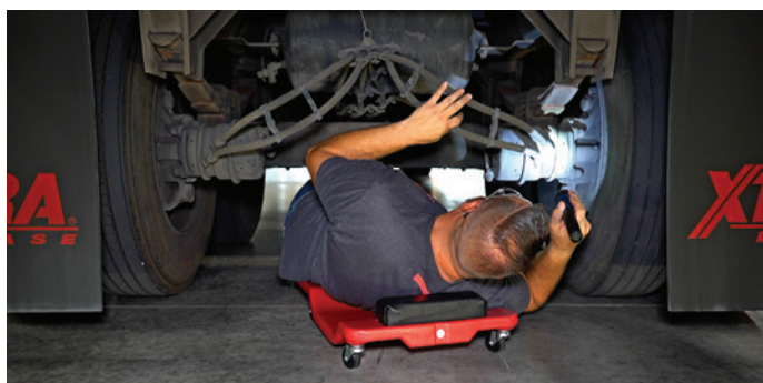
Figure 2. CVSA certified ADS inspector measuring brakes on a Kodiak ADS-equipped CMV
