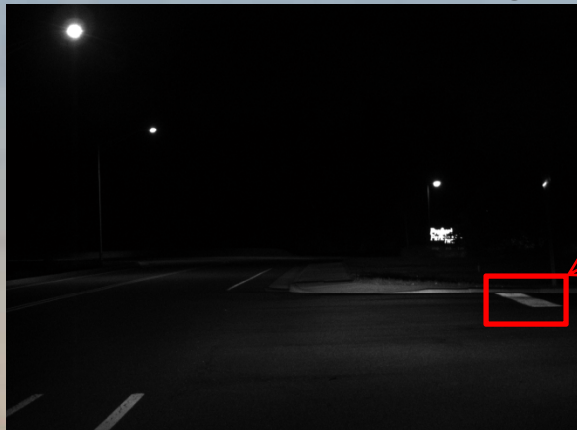
Luminance Camera image (Gain = 0dB, Shutter = 26ms) →
