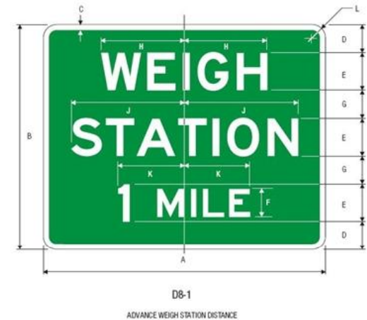
DOT, FHWA D8-1 "Weigh Station" Sign
