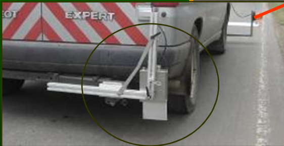
Long Profile and texture (laser + accelerometer)
