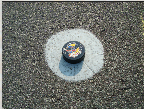
ASTM E965 (“Sand Patch”) – MTD
