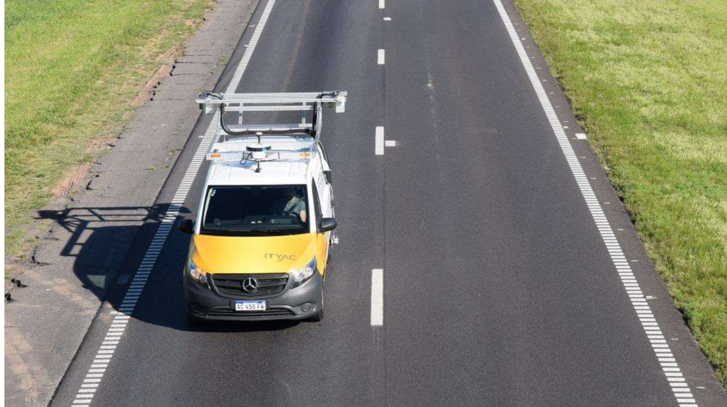
SPIDER™ Multifunction System – Laser Crack Measurement System (LCMS)
