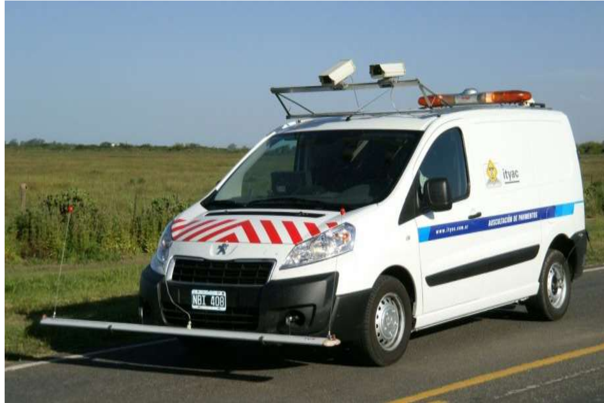
ASTRA™ Multifunction System – Laserprof IRI and Tx – Ultrasound Transversoprofilometer (TUS)
