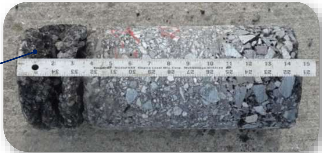
Core 1 (Failed area)
