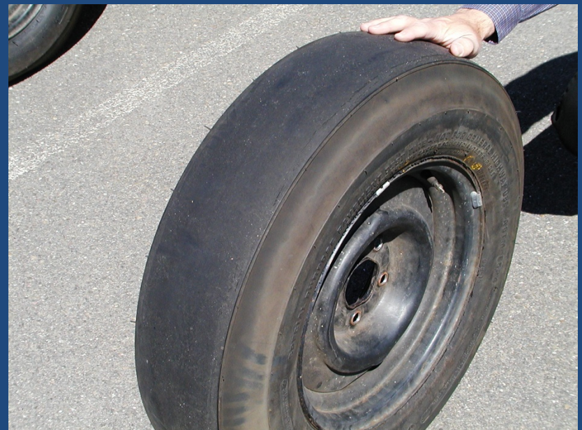
ASTM E 524 Standard Smooth Tire – Relates to Pavement Macro-texture ( 0.02 < \lambda < 2 inches)
