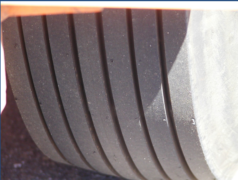
ASTM E 501 Standard Rib Tire – Relates to Pavement Micro-texture ( \lambda < 0.02 inches)
