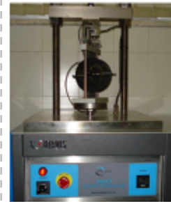
Simplified fatigue life machine “ANAS”
